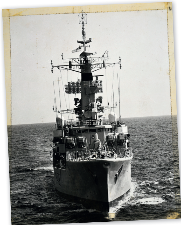
ABOVE THE LEANDER-CLASS FRIGATE 'ARGONAUT'. THE FOUR LAUNCHERS ON HER BOW ARE FOR EXOCET ANTI-SHIP MISSILES (WHICH REPLACED HER MAIN GUNS) AND WERE FITTED BETWEEN 1976-80 COURTESY OF LORD ASHCROFT
