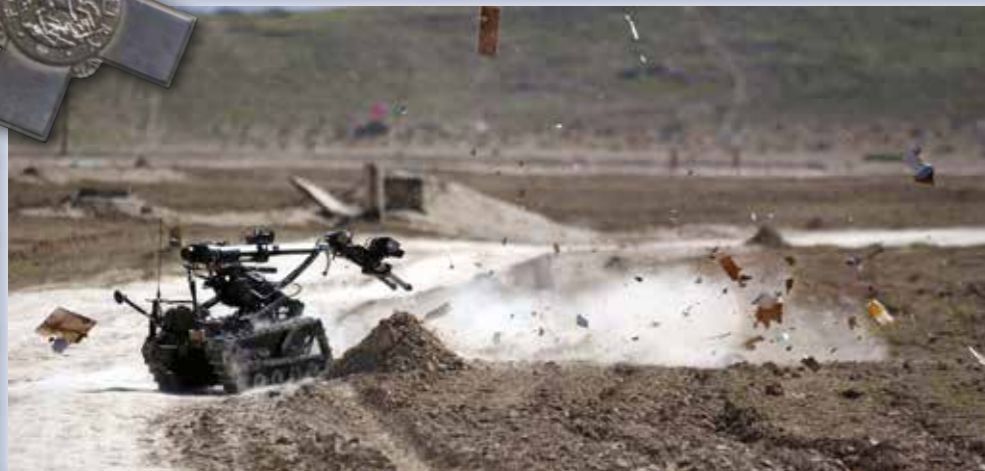
ABOVE: A Royal Logistic Corps Explosive Ordnance Disposal team, part of ISAF's forces in Afghanistan, remotely detonate a suspect explosive device using the Wheelbarrow Mk.8b Bomb Disposal Robot. Able to cross almost any terrain at a speed of up to 6mph, the "barrow" can climb stairs and with an all up weight of 300kg, is more than capable of pushing a saloon car with its brakes applied. (© CROWN/MOD COPYRIGHT, 2014)
